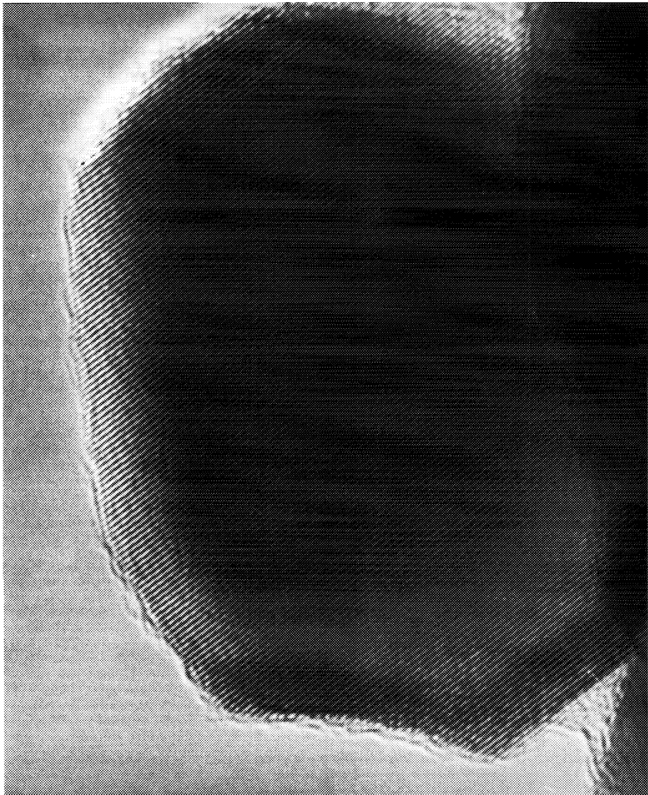
FIG. 2. HRTEM image of a Rh/CeO 2 crystal after reduction at 500°C under H 2 atmosphere (1 cm = 1.625 nm).
